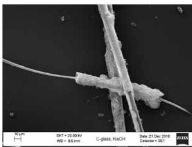
SEM of C-glass shows significant leaching and re-deposition of crystalline deposits.
